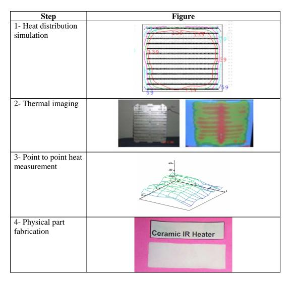
Figure 3. Summary of the heater design for the SIS process
