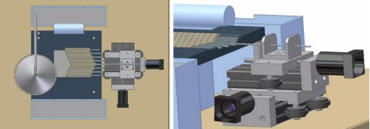
Figure 8. Finger mask system design. A similar mechanism mirror to this mask system will is placed on the other side of the machine.
