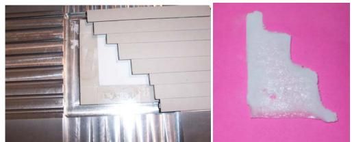
Figure 10. Adjustable fingers and inhibition of sintering in the selected areas
