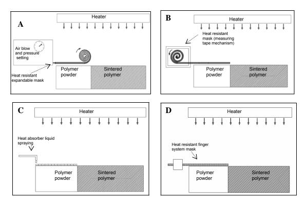
Figure 7. Proposed automated mask systems: A- Air pressure based mask expansion, B-Measuring tape-like expansion mask, C- Heat absorber liquid spraying system, and D- Finger system mask
