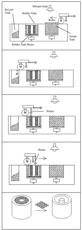
Figure 1. Selective Inhibition Sintering process steps
