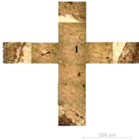
Figure 6: Sections through the micrograph of AL-5 (200 W-120 mms -1 ) generated by 67 Jmm -3
