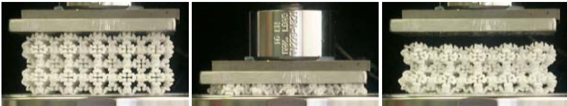
Figure 13- Compression of a helical strut sample
