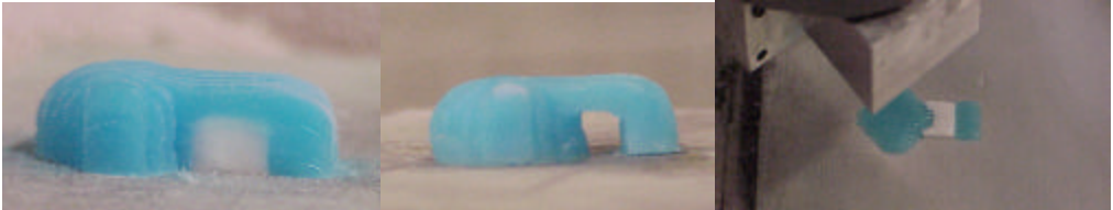
Part C: Ice part with support material (left), after removal (center) and during build (right)
