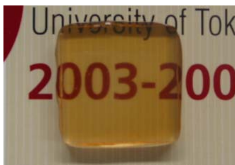
Figure 3 : A Part processed out of CastForm PS after infiltration with UV curable epoxy. This treatment could lowered the haze of the test piece of 5mm in thickness to 55% at minimum.
