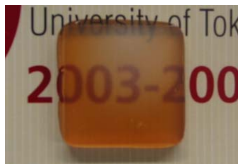
Figure 4: Result of not uniform UV exposure. Clarity and color vary a lot if the exposure is not uniform.
