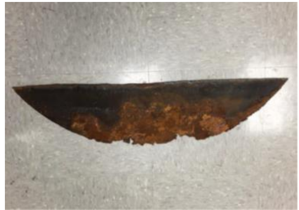
Fig. 2 Failed oil separator weir plate.
