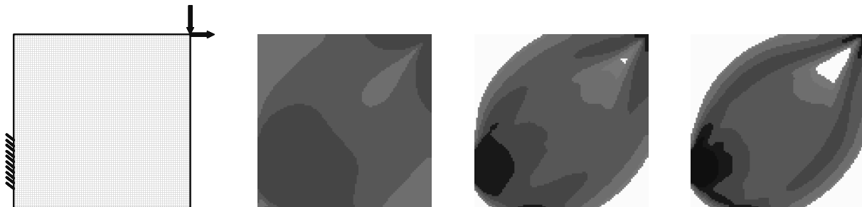
Figure 1. Topology optimization: the cantilever is fixed at the lower left corner; vertical and horizontal loads are placed at the upper right corner. High density regions are darker.
