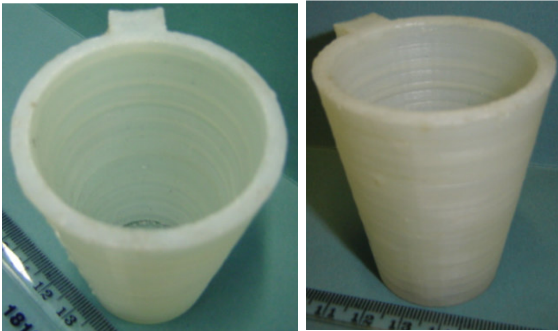
Figure 6: Two views of a cup made for the experiment with the ABS plastic shell.
