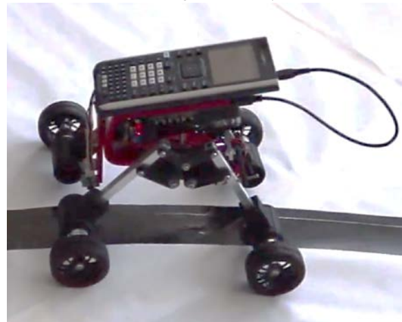
Fig. 3 TI Nspire-Controlled, Line-Follower DSTR
