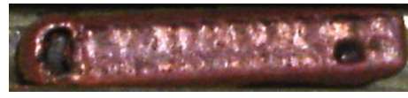
Figure 17. Specimen #12, laser power 66 W, Vs 22,7 mm/s, beam overlap 57%, Vt 0,92 mm/s, T_{avg} 568 °C, scan time 22 s. Layer thickness 1 mm.
