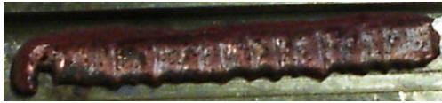
Figure 12. Specimen #3, laser power 66 W, Vs 20,1 mm/s, beam overlap 48%, Vt 0,94 mm/s, T_{avg} 499 °C, scan time 32 s. Layer thickness 1 mm.
