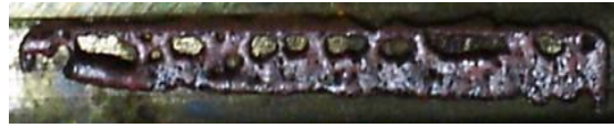
Figure 13. Specimen #4, laser power 66 W, Vs 19,3 mm/s, beam overlap 48%, Vt 0,94 mm/s, T_{avg} 480 °C; scan time 33 s. Layer thickness 0,5 mm.
