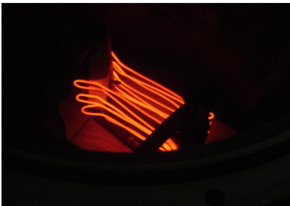
Figure 7. Array of Kanthal™ heating elements glowing inside of the processing chamber.
