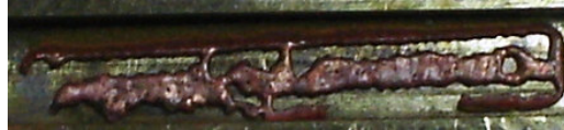
Figure 15. Specimen #6, laser power 66 W, Vs 19 mm/s; beam overlap 48%, Vt 0,88 mm/s; scan time 34 s. Layer thickness 0,5 mm.
