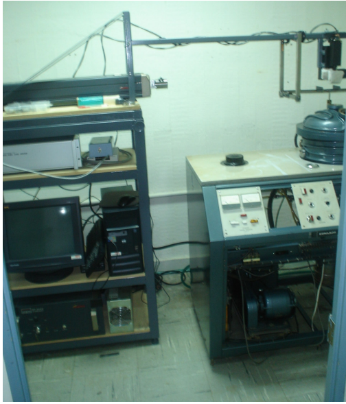
Figure 3. DMLF system showing CO 2 laser unit 80 W SYNRAD, an Edwards vacuum and temperature furnace, Cambridge Technology galvanometric mirrors.
