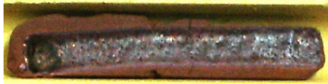
Figure 14. Specimen #5, laser power 66 W, Vs 20 mm/s, beam overlap 48%, Vt 0,89 mm/s, T_{avg} 498 °C, scan time 32 s. Layer thickness 6 mm.
