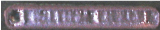
Figure 18. Specimen #17, laser power 66 W, Vs 17,8 mm/s, beam overlap 48%, Vt 1,2 mm/s, T_{avg} 660 °C, scan time 25 s. Layer thickness 1 mm.
