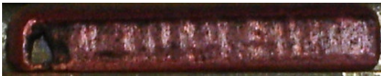
Figure 16. Specimen #7, laser power 66 W, Vs 19 mm/s, beam overlap 48%, Vt 0,89 mm/s, T_{avg} 498°C, scan time 33 s. Layer thickness 1 mm.
