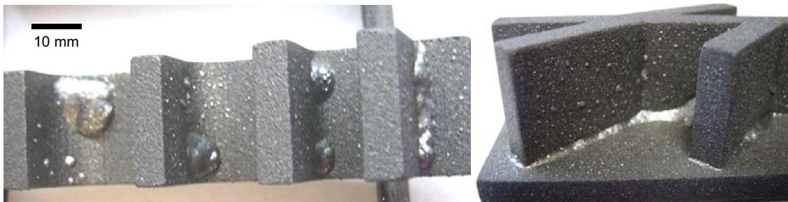
Figure 5: Macroscopic Overfilling at Geometrical Stress Concentrations
