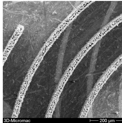
Fig. 5b: Top view of a coiled tungsten ligament (height: 300µm); the cut-ins from the pulses are clearly visible.
