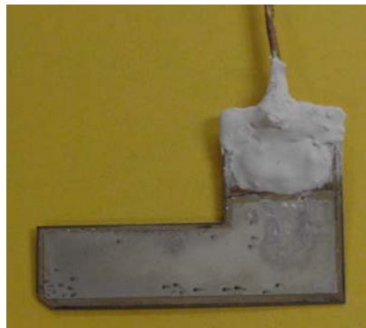
Figure 4. Image of a TFTC with cemented connection
