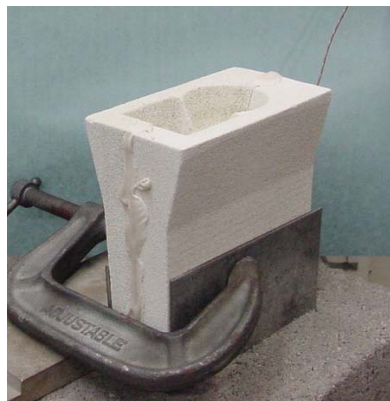
Figure 5. Image of 3DP mold with TFTC connected to the NI 6070E DAQ system prepared for casting
