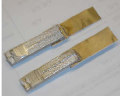
Figure 3. Lap joint test bars before testing
