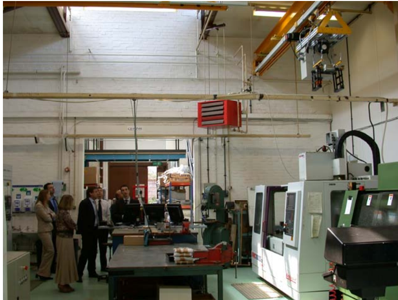
Figure 5: A photograph of the finished FASTOOL grabber and trolley in action. The commands are being relayed via a Windows PC in another room of the building.
