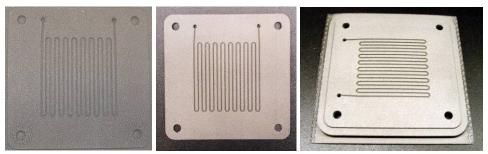
Fig.6. Sample plates created with the TS-3DP method
