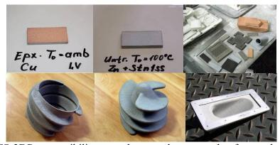
Fig.2. Initial TS-3DP compatibility test tokens, and an example of a net-shaped metal part.
