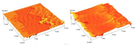
Fig. 10. (a) Current (in pA) on the scanned surface at 1V bias potential, (b) Surface topology.
