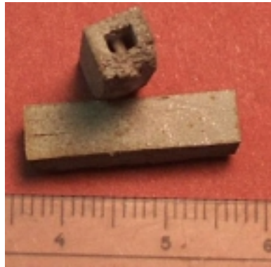
Figure 8. Sintered and reduced trussed channel test sample
