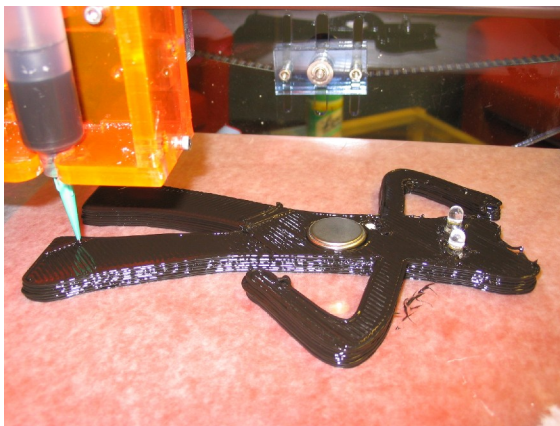
Figure 19 – Holes are left to accommodate the LEDs and the battery.
