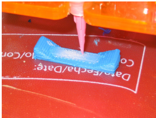
Figure 13 – Silicone printed on top of a frosting support.
