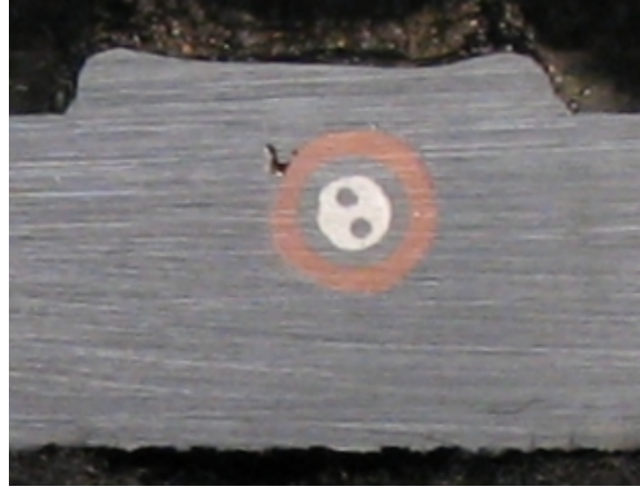
Figure 4: Cross section of embedded K-type thermocouple.
