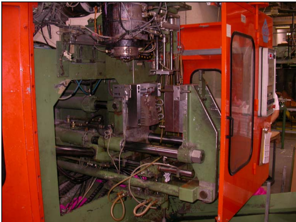
Figure 13: DMLS mould tool part in place in the blow moulding machine
