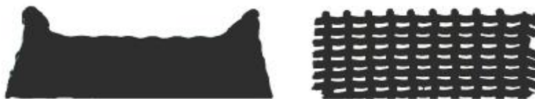
Figure 3: Vertical cut of plotted polyurethane scaffolds. The left scaffold was plotted in air, while the right one was plotted in a plott medium (water).
