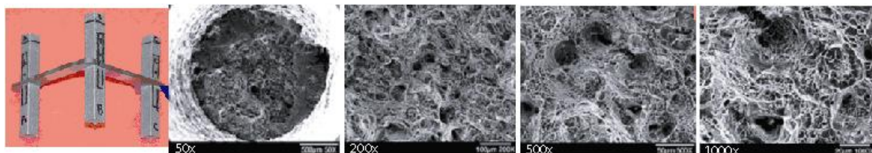
Figure 12. Fracture Surface of a Type M LENS Build on Both Sides of a Wrought Substrate.
