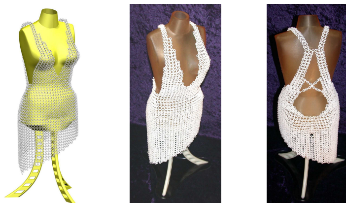
Figure 5: World's first 3D conformal RM textile garment, designed by Guy Bingham, CAD model (Left), actual garment (Centre & Right)
