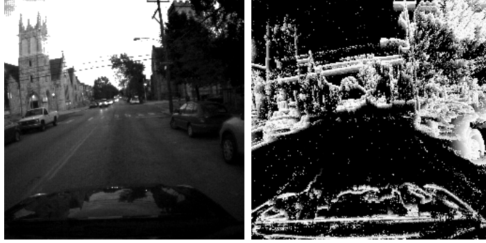
Figure 25: Example of a timestamp image. Left: Grayscale output. Right: Timestamp image, where each pixel represents the timestamp of the most recent event. Brighter is more recent.
