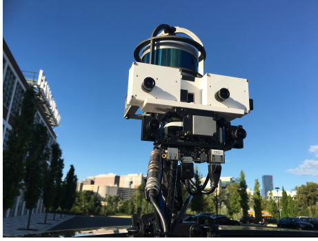
Figure 14: Full sensor rig, with stereo DAVIS cameras, VI Sensor and Velodyne lidar.
