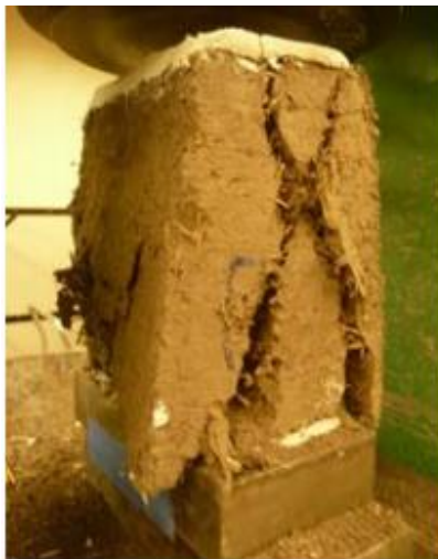
Figure 2.1: Compressive Strength Failure
