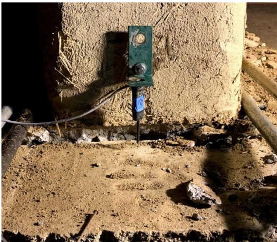
Figure 6.11: Foundation at Failure
