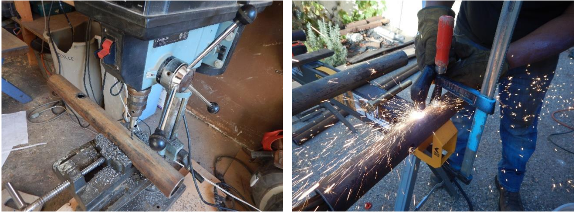
Figure 4.2: Fabrication of the Recycled Steel Reinforcement
