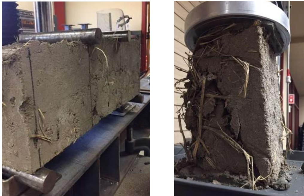
Figure 2.9: a) Modulus of Rupture Test Setup b) Compression Test Setup
