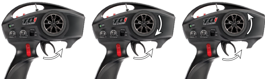
Figure 8.4: Fault trigger commands: temporary fault (left); temporary fault with soft reset (center); latched fault (right).
