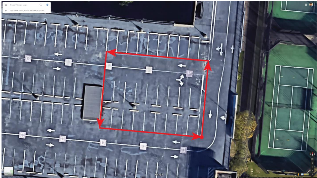
Figure 44: Counter-clockwise rectangular travel path. The long leg of travel is approximately 28 m, and the short leg of travel is approximately 22.5 m. Map data © 2018 Google. Reproduced with permission from Google Maps Geoguidelines, 2019 [123].
