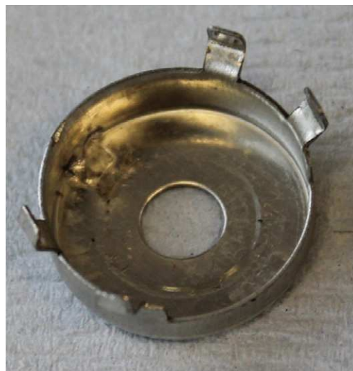
Figure 5. The base of the potentiometer with the lug hammered out to allow 360° rotation.
