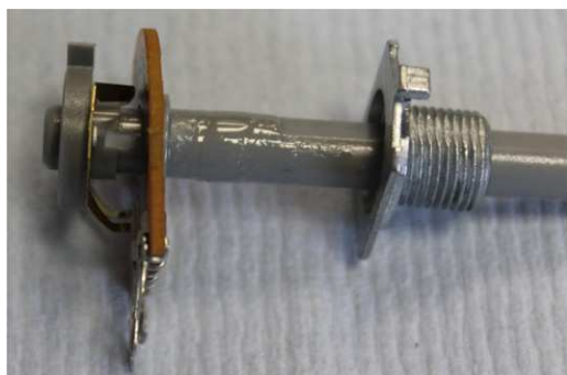
Figure 7. Lubricated spindle of the potentiometer to allow smooth and even rotation.
