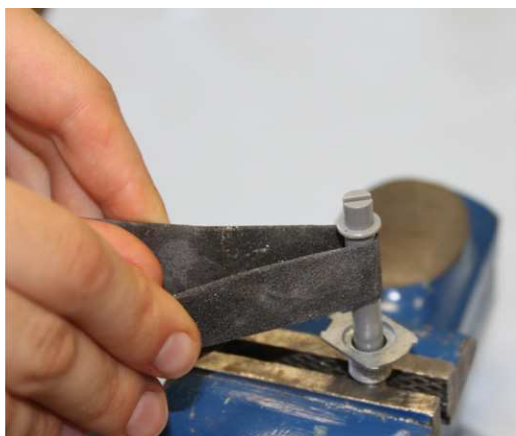
Figure 8. The potentiometer spindle should be sanded down to an appropriate diameter to allow smooth 360° rotation.
