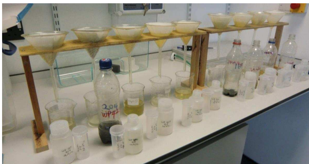
Plate 4.2 Filtration process and equipment
