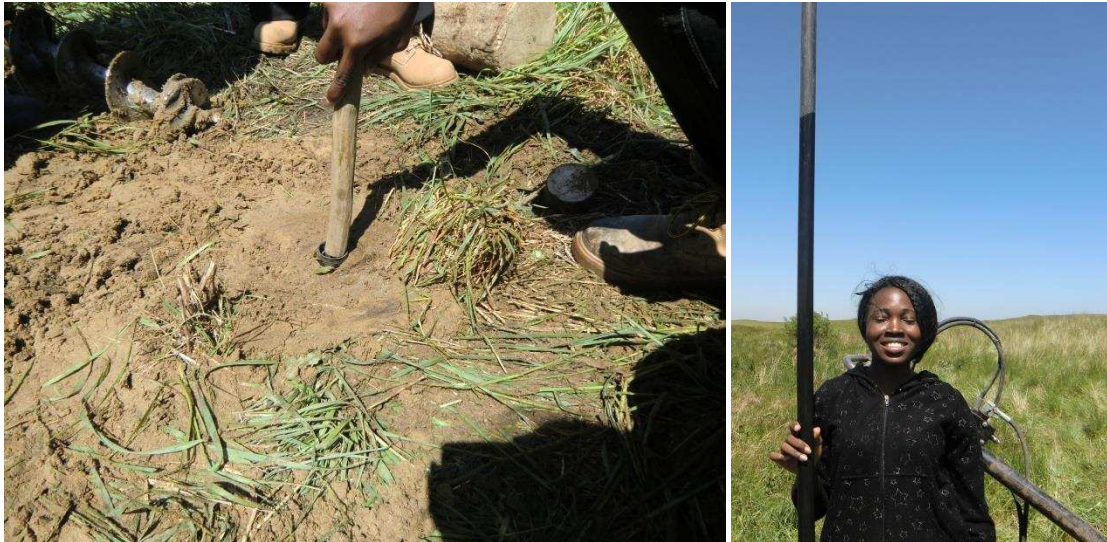
Plate 3.3 Internal 32mm diameter sheathing pipe being removed from the dipwell and visual water table level observation
