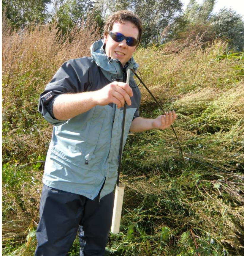
Plate 4.1 Dipwell sample collection using bailer
