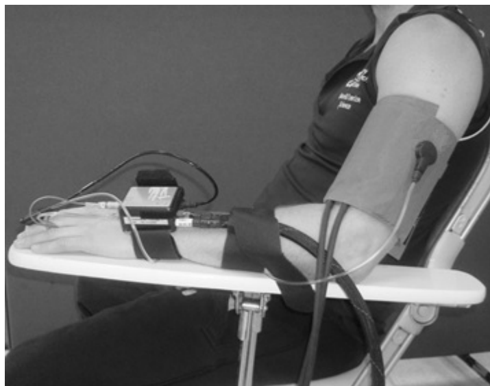
Figure 2.5. The setup of the Finometer finger cuff, height correction unit, front end box and upper arm cuff.
