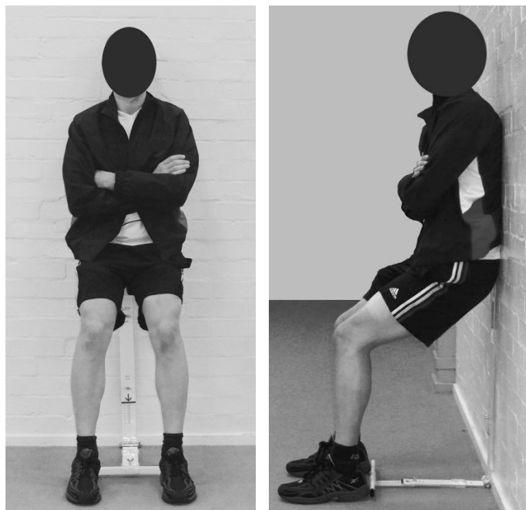
Figure 2.12. The Bend and Squat device for setting knee joint angle during isometric wall squat exercise.
