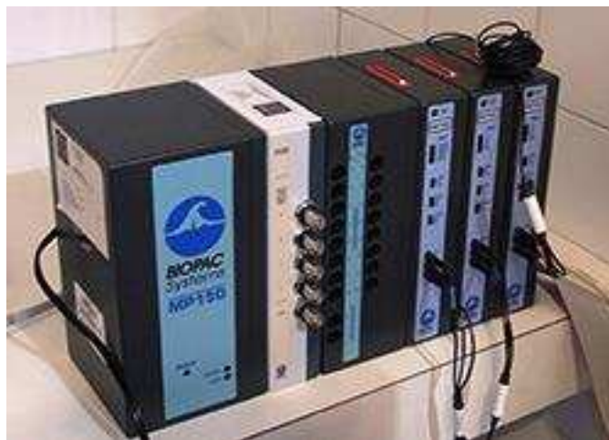
Figure 4.4: BIOPACK ® MP150A-CE system, with adjacent SKT100C and HLT100C modules
