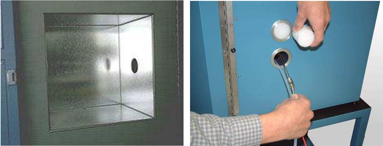
Figure 5.4: Access port plug of the 2500 Humidity Chamber
