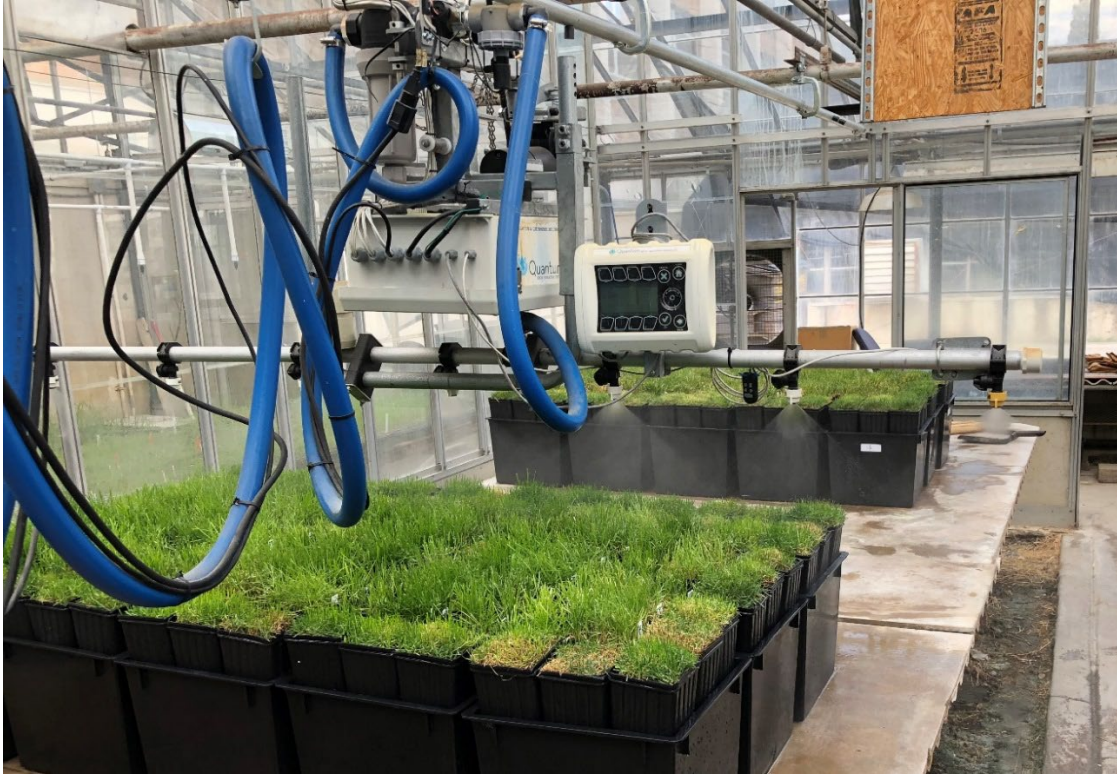
Figure 1. Greenhouse arrangement of entries with the boom sprayer that applied control and salt irrigation treatments.
