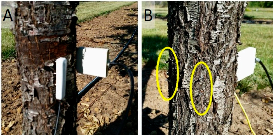
Figure 2. (A) GS3 and CS655 installed in a peach tree trunk revealing some exposed waveguide near the sensor head. (B) CS655 and TDR-315(L) sensors protruding through a peach tree trunk.
