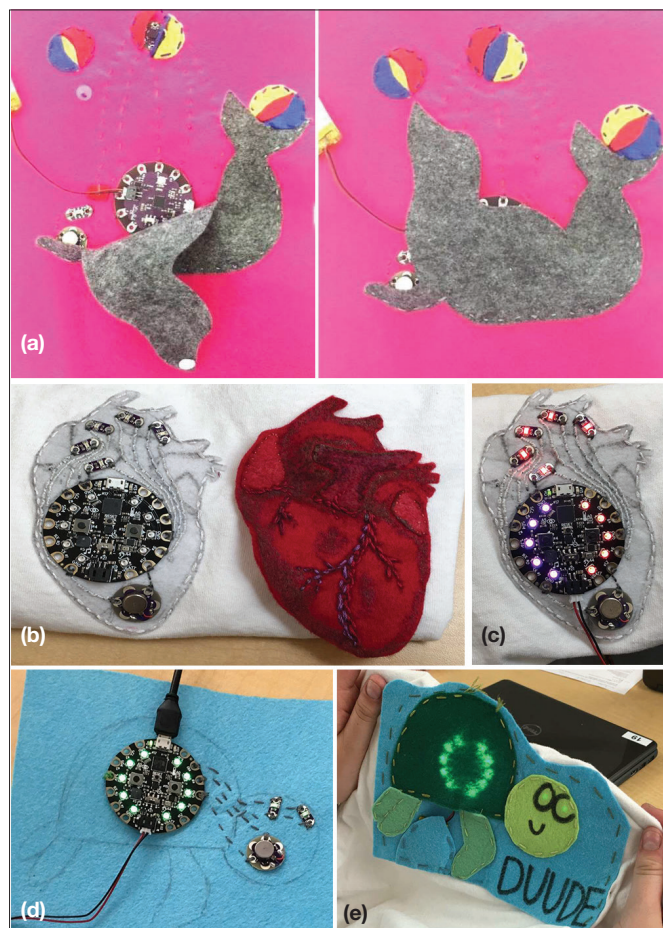
Fig. 1. (a) “Slouch-sensing” e-shirts sewn with an Arduino Lilypad (b) and (c) Adafruit Circuit Playground, (d) an accelerometer, a buzzer, and LEDs, and (e) an artistic design cover.
