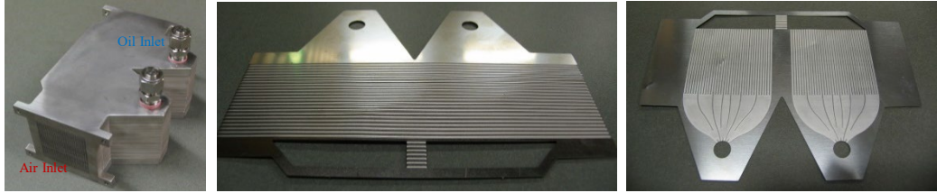
172 Figure 4. (left) A photograph of the HRU showing air and oil inlets; (middle) Exhaust shim; (right) 173 Oil shim
