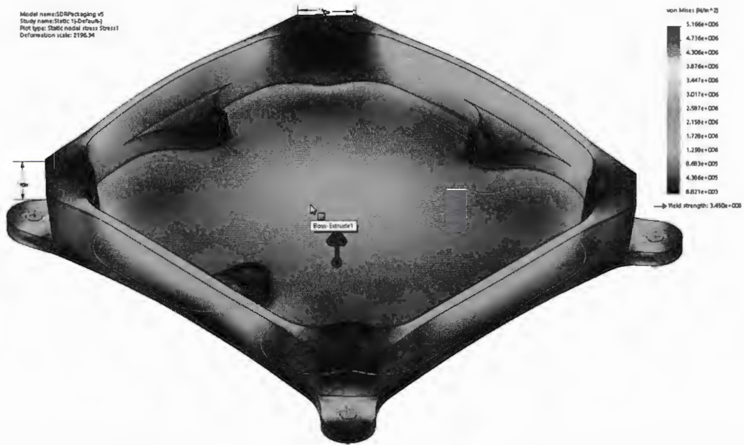
Figure 22: Stress distribution in the packaging base for a 60g acceleration load applied in the positive y direction
