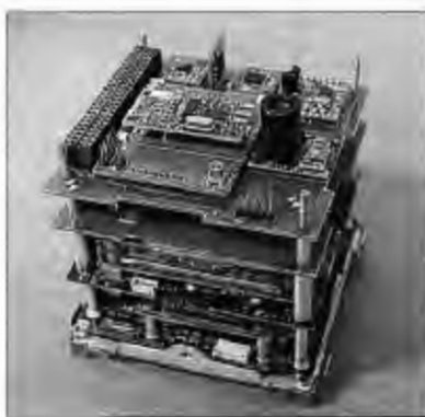
Figure 8: Typical CubeSat board stack
