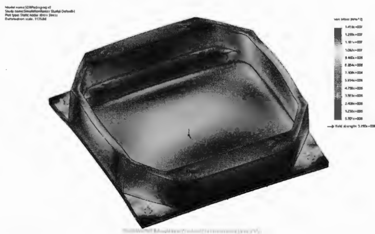
Figure 17: Stress distribution for the z-axis static loading study of the initial packaging base
