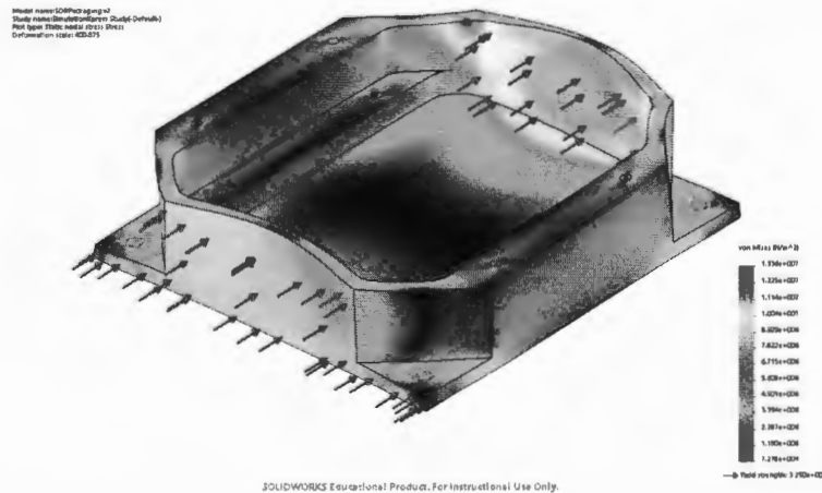
Figure 15: Stress distribution for the x-axis static loading study of the initial packaging base
