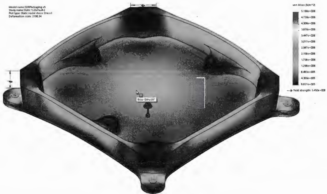
Figure 21: Stress distribution in the packaging base for a 60g acceleration load applied in the negative x direction
