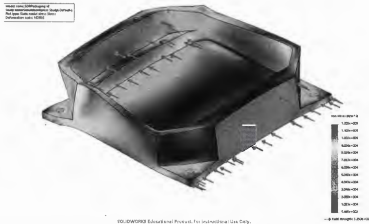
Figure 16: Stress distribution for the y-axis static loading study of the initial packaging base
