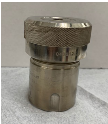
Figure 1.1: Photo showing the autoclave reactor used for carrying out solvothermal syntheses.
