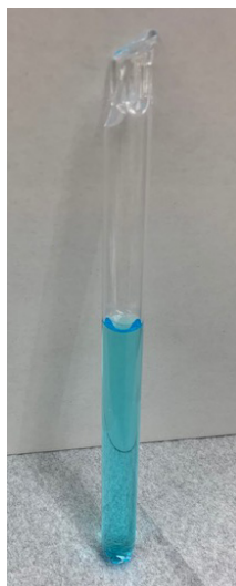
Figure 1.2: Photo showing a fused silica tube with solution sealed within for solvothermal reactions.
