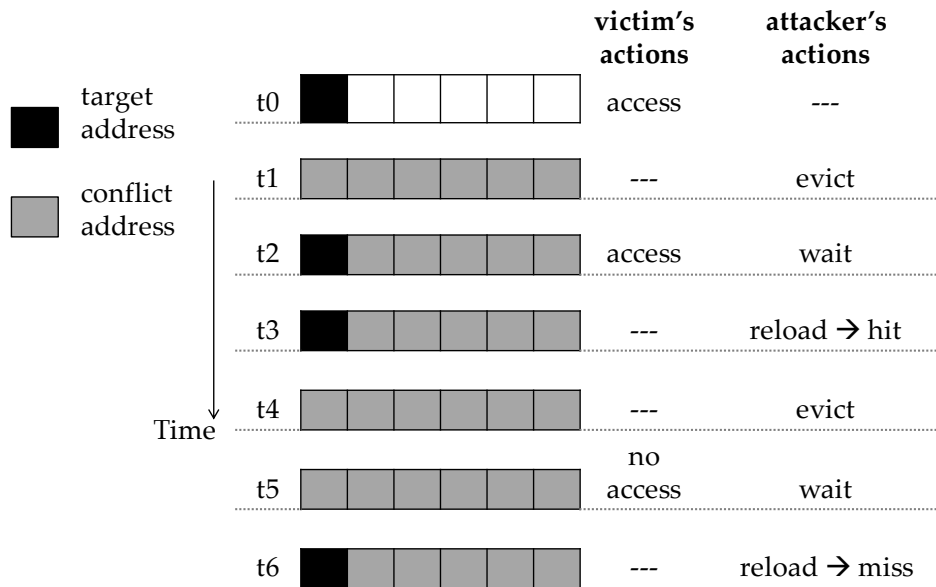
Figure 2.3: Evict+reload attack example.
