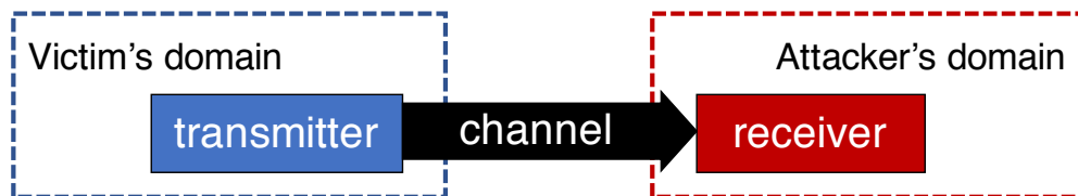
Figure 2.4: Cache attack schema involves two procedures: 1) the transmitter changes cache states in a secret-dependent way; and 2) the receiver detects the cache states and extracts the secret.
