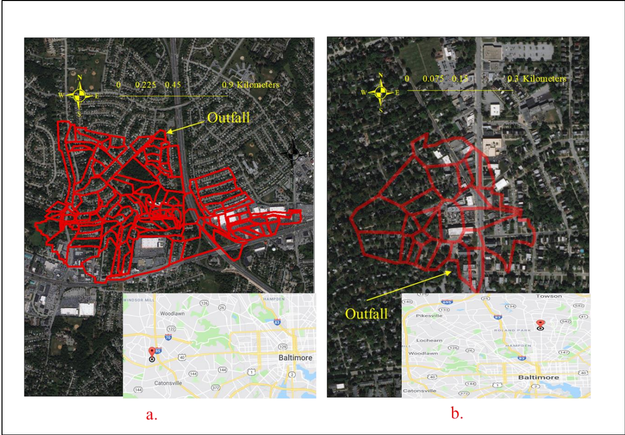
Fig. 2.1. Boundaries of the modeled (a) DR5 and (b) SR5 watersheds in the state of Maryland, and their subwatersheds modeled in SWMM 5.0, along with their relative locations
