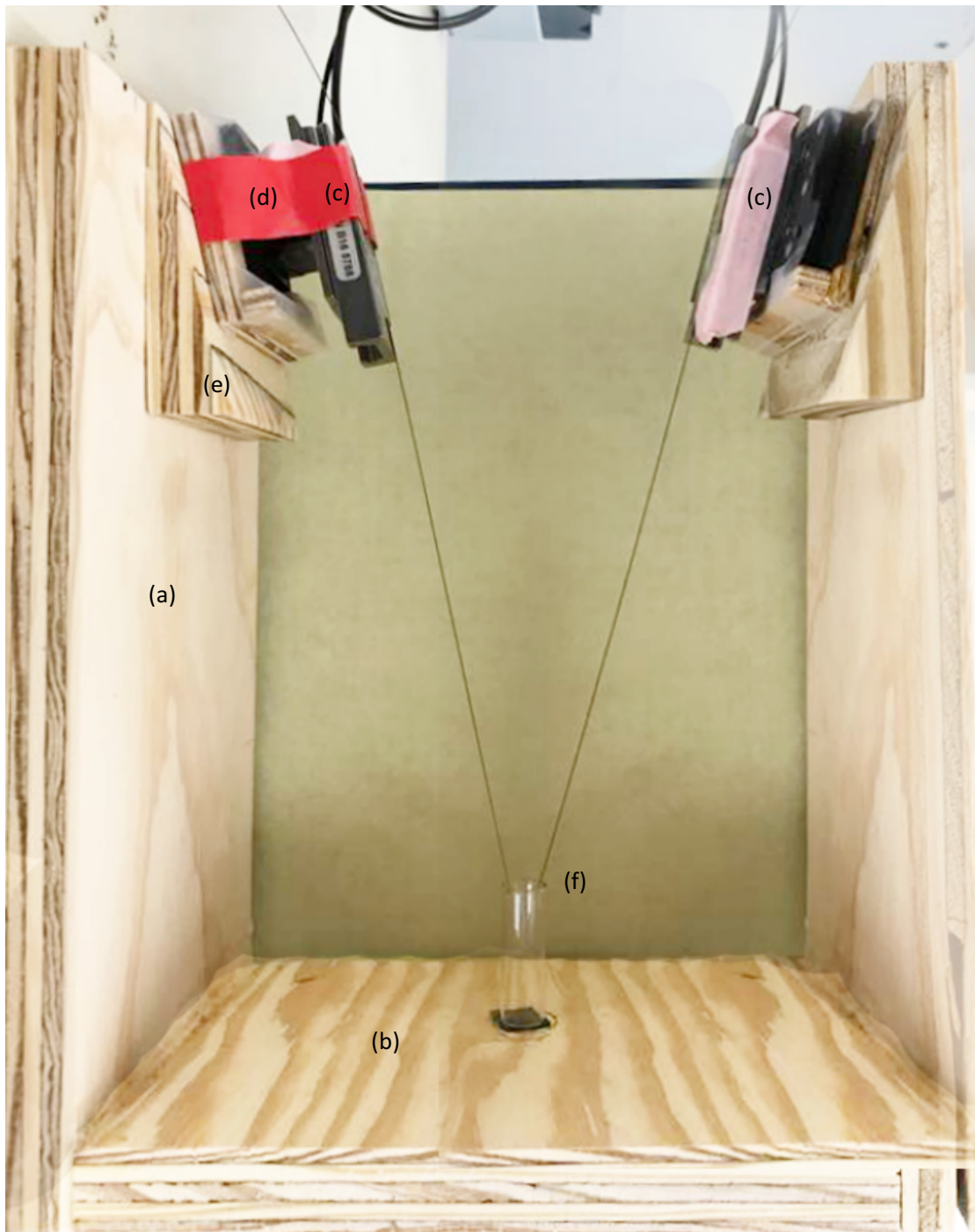
Figure 32. Assembly of the wood stand's (a) walls (b) base (c) micromotors to translationally move the polymer- and cargo-carrying tubes (d) a goniometer to control the precise injection of the cargo within the microbubble (e) angled wood stands for attaching the micromotors to the walls and (f) a sample of a glass vial.
