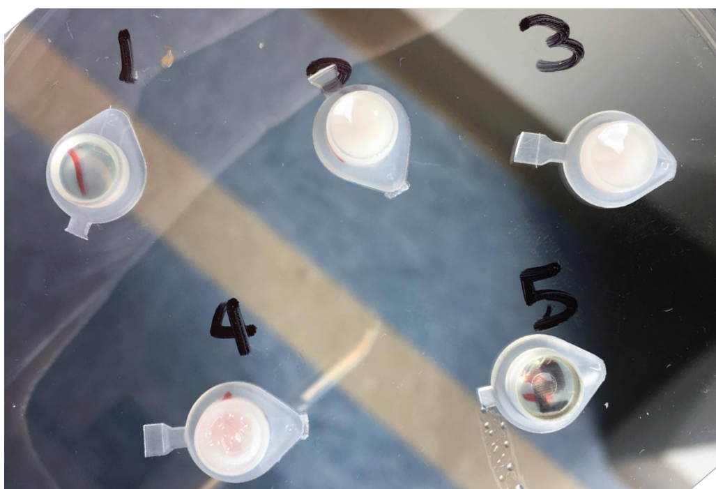
Figure 14 PCLTA polymer with different ratios after UV curing (1) PCL:PCLTA=1:0 (2)PCL:PCLTA= 1:1 (3)PCL:PCLTA= 1:3 (4) PCL:PCLTA= 3:1(5) PCL:PCLTA= 0:1.
