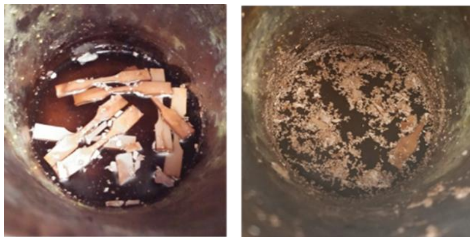
Figure 3.9. Images of the PEEK specimens in the vessel, treated with fluid 3 for 21 days (left) and 28 days (right).
