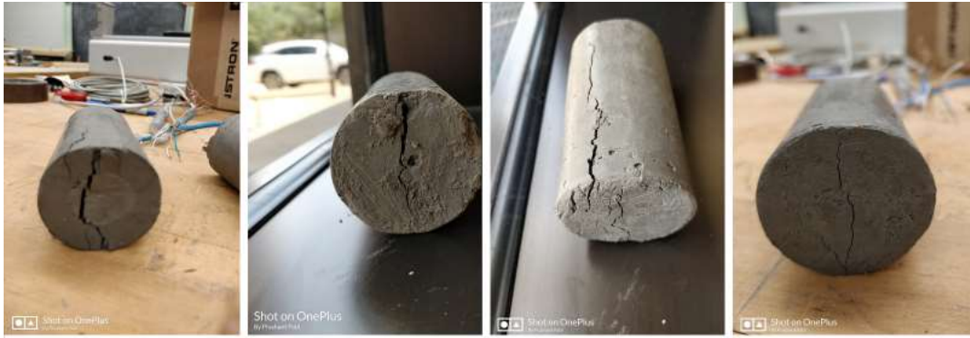
Figure 5 Specimen Failed in Split Tensile Test
