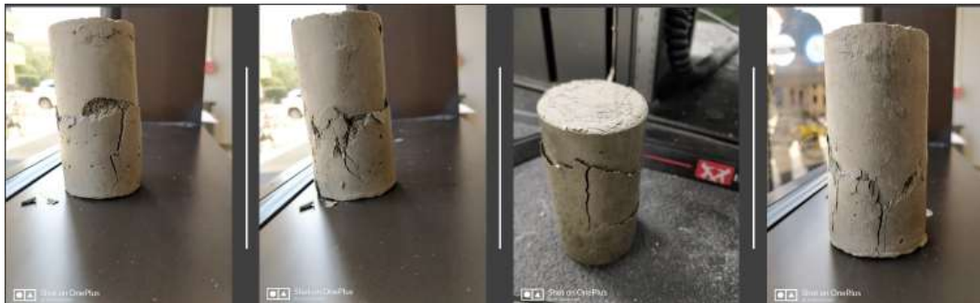
Figure 4 Specimen Failed in Unconfined and Confined Compression Test
