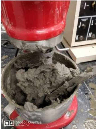
Figure 2 Soil and Grout Mixing in a Mixer
