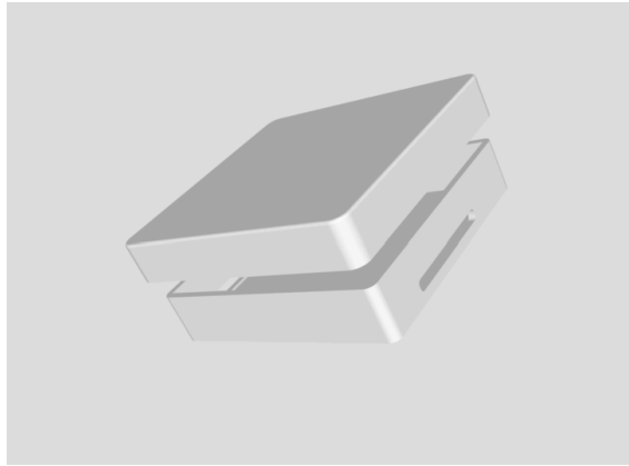
Figure 2: Autodesk Fusion 360 (STV) model of the 3D Printed Case
