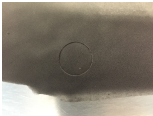
Figure 21: Electrode sheet shown with punched cathode
