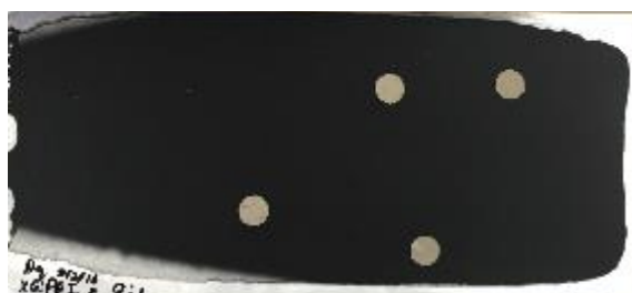
Figure 47: Aqueous sheet dried at 50°C with 9% XG and 1% PEI by mass
