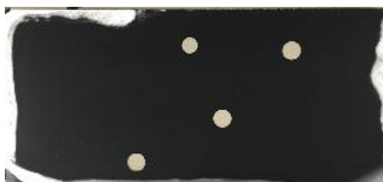
Figure 46: Aqueous sheet dried at 50°C with 8% XG and 2% PEI by mass
