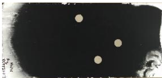
Figure 45: Aqueous sheet dried at 50°C with 7% XG and 3% PEI by mass
