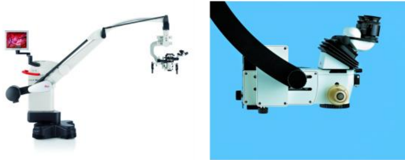
Figure 3.6: Leica M400E Surgical Microscope. The arm balances the microscope over the patient and is manually positioned by the operator. Fine-focusing is then used to precisely place the focal plane.
