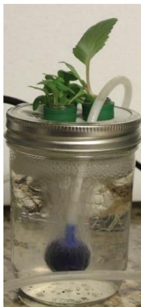
Figure 56. Hydroponic system for cabbage exposure to yttria NPs
