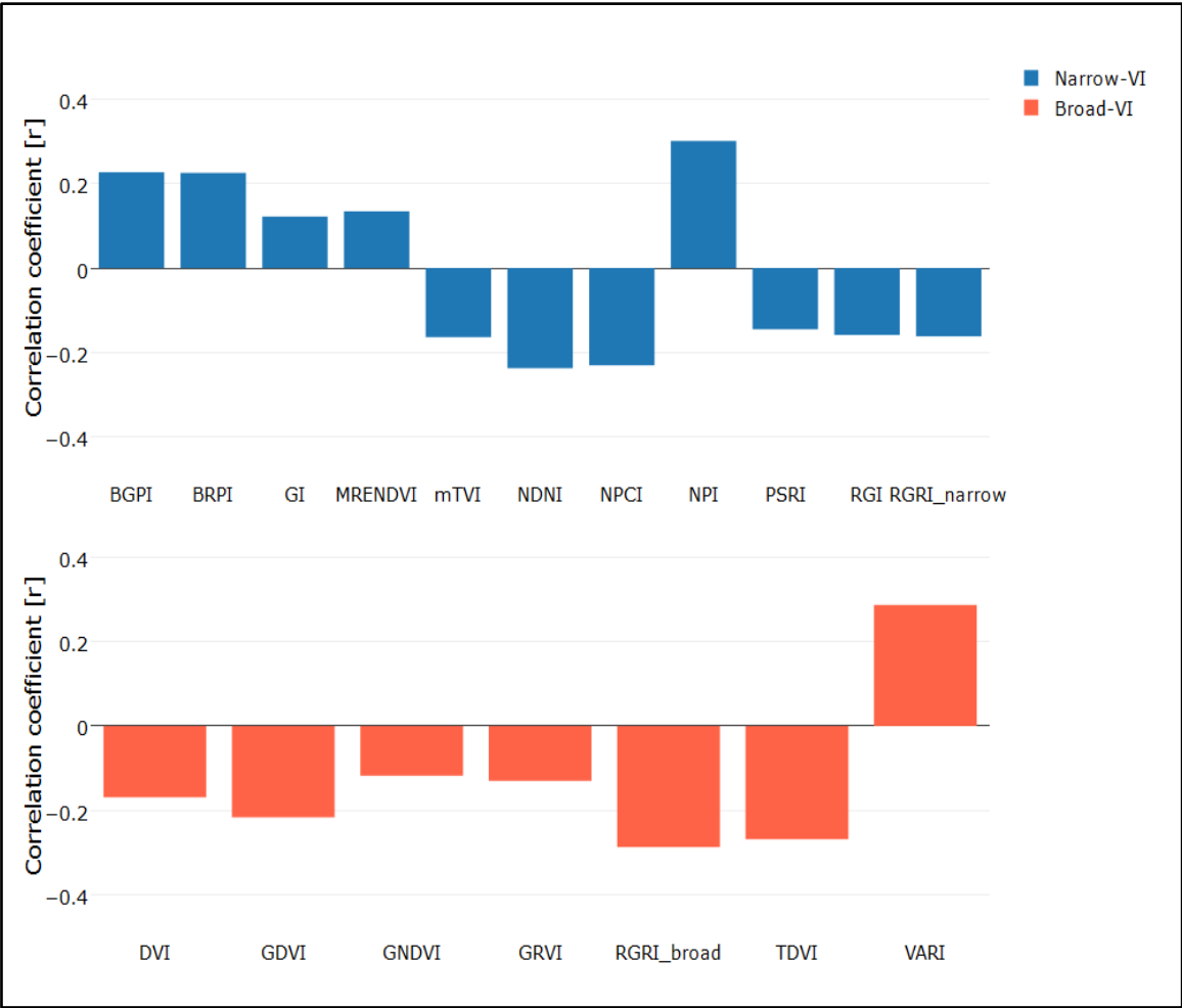
Fig. 19 Pearson correlation coefficients of the EW load and the narrow and broad vegetation indices (VI).
