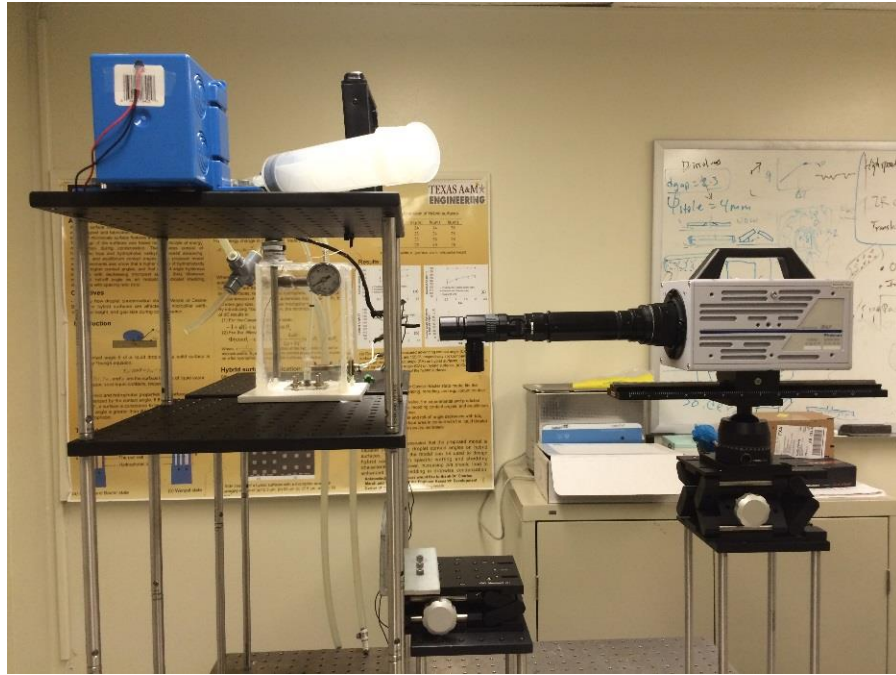
Figure 16. Side view of flow rate and quality measurement pump assisted system
