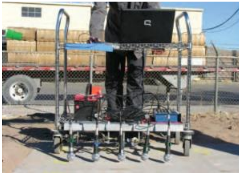
Figure 2.8: Impact-Echo Device University of Illinois Urbana-Champaign (Gucunski et al., 2013)
