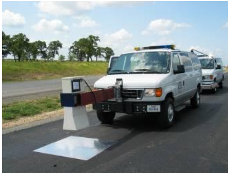
Figure 2.2: Air-Coupled GPR System (Wimsatt et al., 2008)
