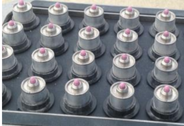
Figure 4.6: Rubber Securement In-between Transducers
