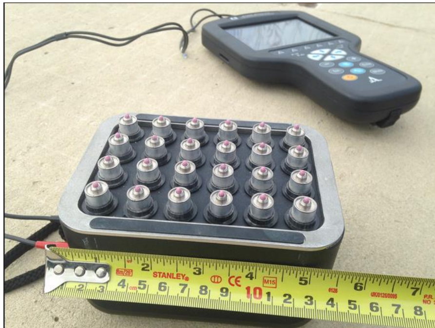
Figure 2.14: Transducer Array (Foreground) with EYECON Handheld Computer (Background)
