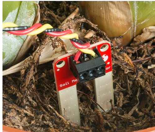
Figure 3.5: Soil moisture sensor installed in the field for acquiring soil moisture content data.
