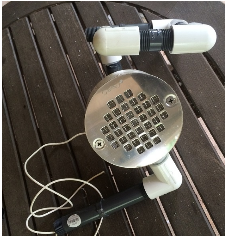
Figure 3.2: Second-generation runoff sensor is equipped with a mesh like filter to filter out mud and debris.
