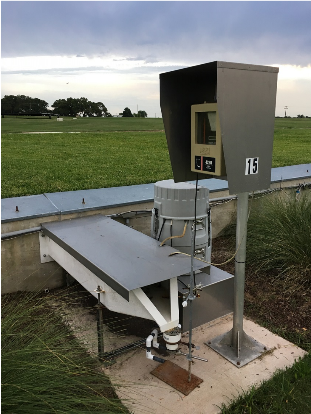
Figure 4.1: Flowmeter setup in the runoff field laboratory to collect the runoff flow data which is further used for analysis purposes.
