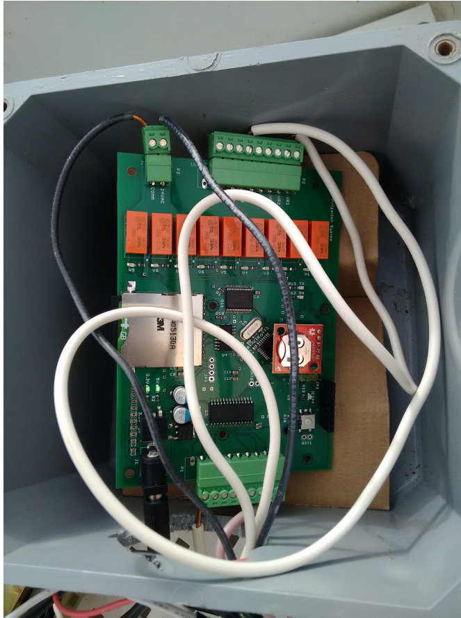
Figure 2.2: Controller unit used in First-generation LIRMS. The operational logic discussed in 2.1 is implemented on the controller unit.
